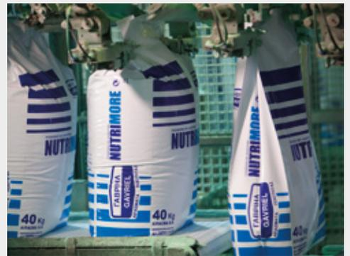
When fed into the filling machine, the tubular FFS film is base-sealed and cut, formed and filled, and then top sealed. The same procedure applies for the flat FFS film, with an extra phase for vertical sealing before base sealing.
